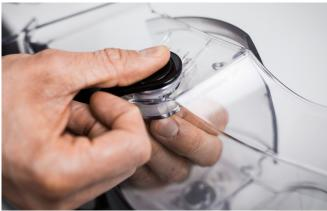
6. Push shutter in the direction opposite of the nozzle until the shutter's holes overlap with handle's holes. Click plugs into the holes in the sides of front, securing the handle to the front. Do this for both plugs. Make sure you hear one click per plug being attached - if not, keep trying by pushing the front and the shutter together using both hands as shown in the right picture above.
