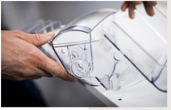
3. Lay bin front on a flat surface. Grab shutter. There are four pegs on the shutter in total - the two pegs to which the springs are attached should be the ones closest to you. Insert shutter into bin front with protruding circles entering front first. Push sides of shutter slightly inwards in order to make the shutter squeeze past sides of front. Click protruding circles into the corresponding holes in the sides of front.
