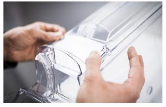
**13.** With bin in the same position, click shutter stop into place in its hinges. Make sure shutter stop is installed in a way that places the encircled plastic grip on inside of the bin.
