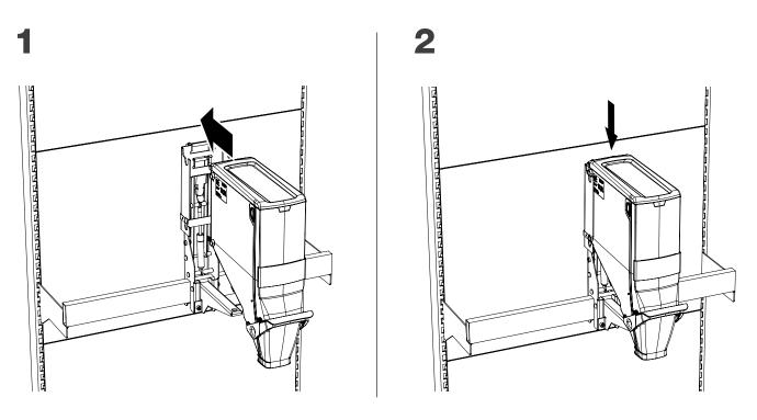
**N.B.** Only pull down one Gravity Bin at a time for refilling. Push it up before taking down the next one. Uprights & X-bars might not be constructed to support the weight if all bins are pulled down at the same time.
