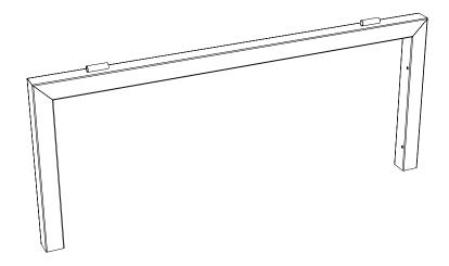
2 Attach the side to the front frame using two bolts
