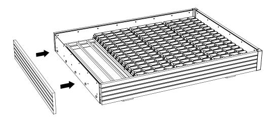
**12** Fix the side panel with six self tapping screws
