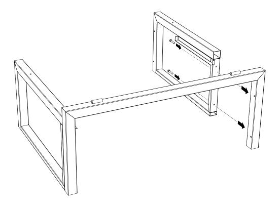
4 Attach the back frame to both sides using four bolts
