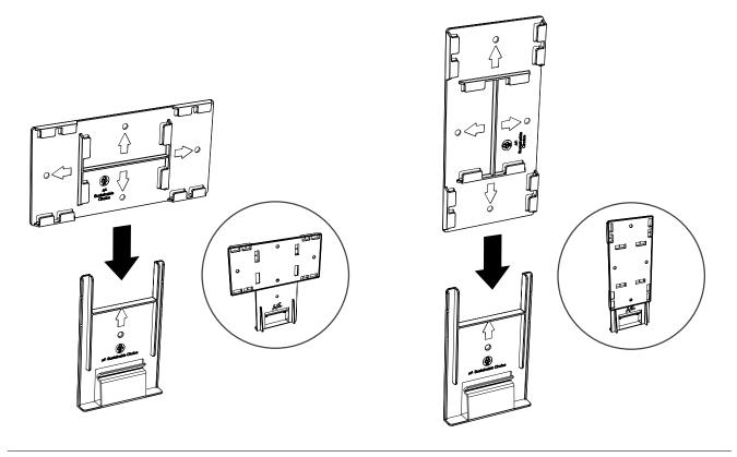
Lock the eXtender plate to the Facer  $^{\text{TM}}$  XL frame.
