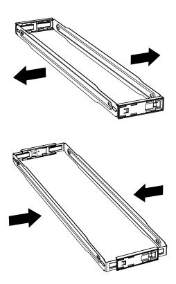
Place the frame behind the front riser. Ensure the Facer<sup>™</sup> front sits in the locking channel for the best fit.
