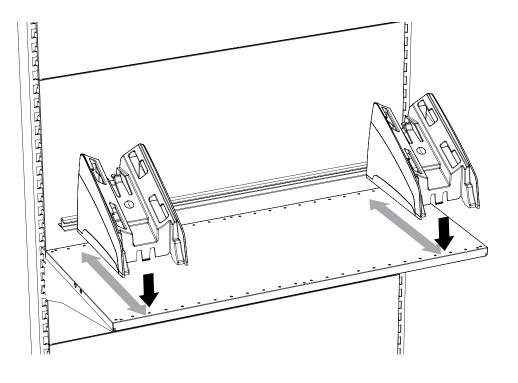
Once the correct depth has been determined, remove the tape and fix the profile to the shelf
