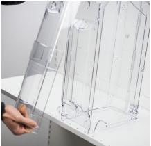
2. Press bin front's latches one at the 3. Remove clip - lift its fly upwards time to separate front from bin body. while pushing clip to the right. Remove bin front.
