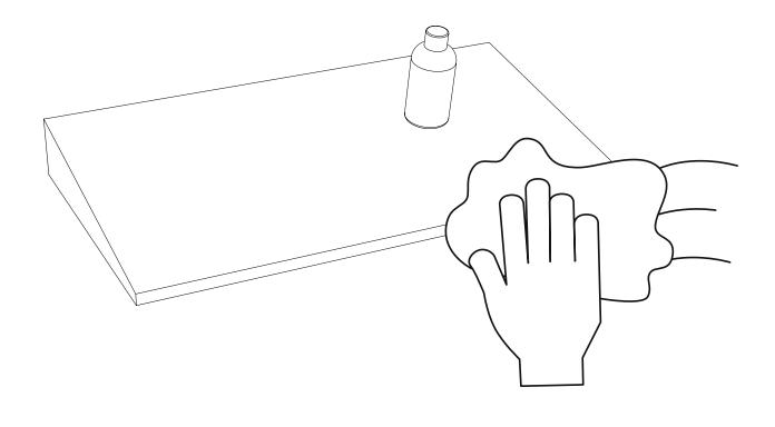
2 Remove the protection film from the front stop, place it at the front of the shelf and press firmly
