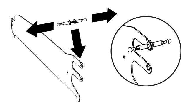
Install stabilizer onto the back of the divider. Note: Dividers on the end (Sides) of the sheet should not have stabilizers.
