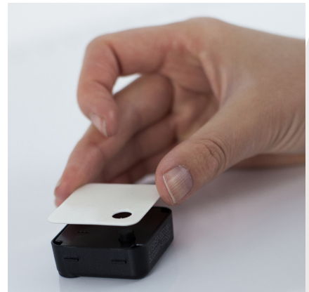
Align hole in adhesive with button on tag
