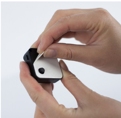
Remove liner from adhesive on base of tag.
