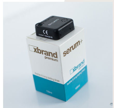
After tag is attached, it will beep in about 10 seconds to indicate it was properly attached. Tag will be dormant for 3 minutes, after which the light and motion sensor are silently activated.
